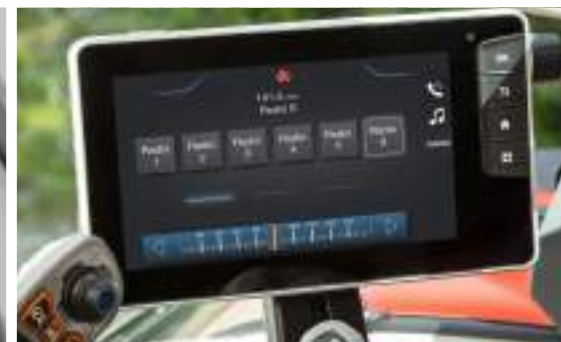
BLUETOOTH RDS/MP3 RADIO is fitted as standard allowing hands-free calls. Optional phone and data radio controls through the Datatronic 5.
